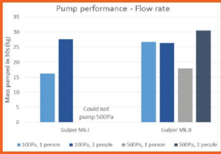
Figure 2 – Results of pump performance testing
