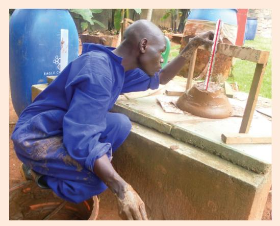
Slump Cone test for shear strength determination
